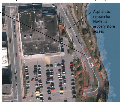
This Vibrancy Project involves the removal of asphalt paving and concrete curb and gutter south of the No Frills driveway off of Water Street. An in-kind contribution by Basterfield and Associates will result in a design drawing and specifications detailing the construction of an attractive landscape and low impact development (LID) storm water management feature in the area. The affected area is shown in the figure below.
