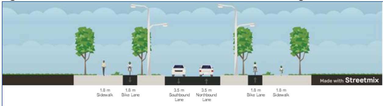
Figure 3: Ashburnham Drive Recommended Cross-Section Design
