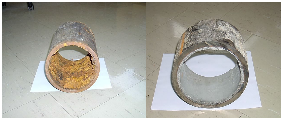
Figure 3: Tuberculated water main and cement lined water main
