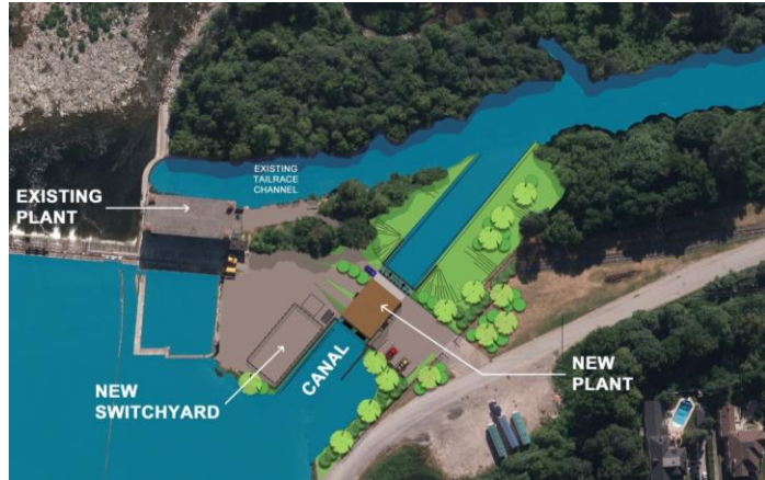
Schematic of the London Street Generating Station Expansion
