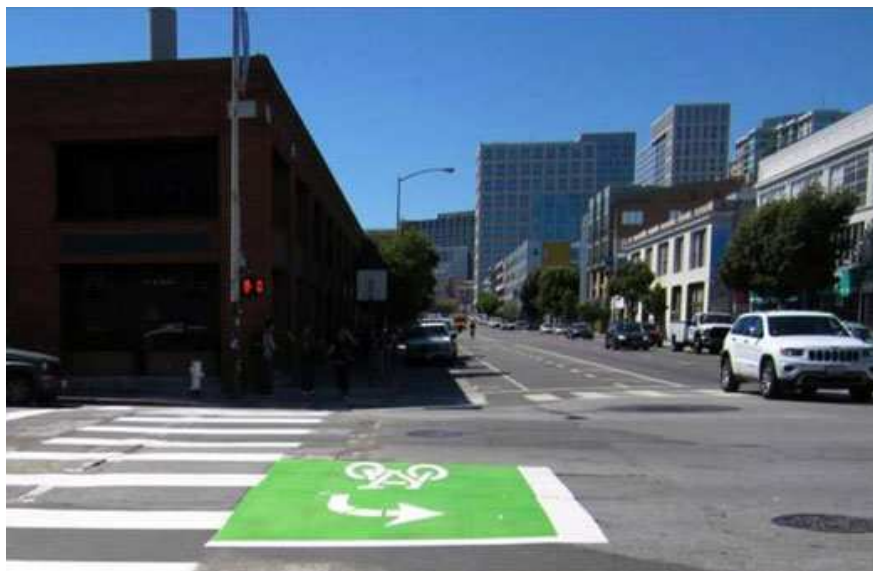
Figure 3.2 – Left Turn Box for Cyclists
