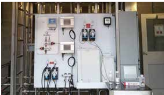
Below: Ozone contactor installed to study effects of advanced oxidation on Otonabee River water
